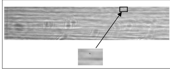
Figure 4: Image of the X-ray beam. The fringes are created by the defects on the windows crossed by the beam and on the monochromator. An example of abnormal pixel is shown in the detail.
