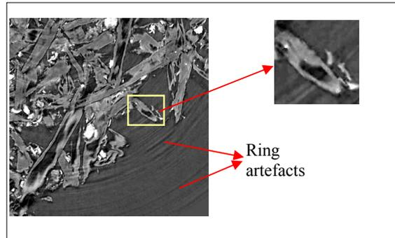
Figure 3: Reconstructed slice of paper. Fibres and fillers (white stains) are designable. In the details, the edge enhancement is shown (dark zone around the fibre).
