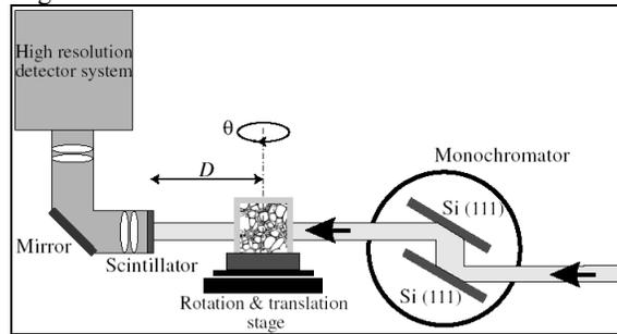
Figure 1: Principle of parallel and monochromatic beam Micro-tomography at beamline ID19 of the ESRF. The synchrotron beam is monochromatised either by a double silicon crystal monochromator or by an  $\text{Al}_2\text{O}_3/\text{Ru}$  multilayer. Radiographs for a large number of angular settings  $\theta$  over a  $180^\circ$  range are recorded with a CCD based high resolution detector system. The sample detector distance  $D$  can be varied from  $\approx 0$  to 1 m.
