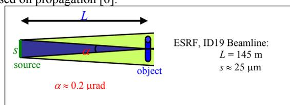
Figure 2: The small size of the electron beam cross section, the small horizontal and vertical (the green zone) divergency of the source ( $< 100 \mu\text{rad}$ ) and large distance between the source and the sample ( $L$ ). This leads to a very small angular extension ( $\alpha$ ) of the source as see.
