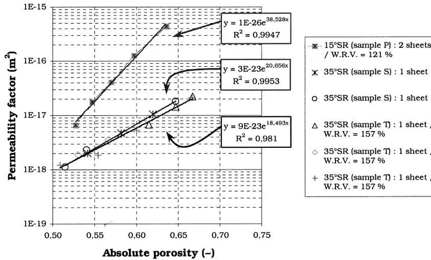
Figure 7. Correlations [a.exp(b.n)] obtained for different samples of softwood pulp (basis weight for all the sheets is  $100 \text{ g} \cdot \text{m}^{-2}$ ).
