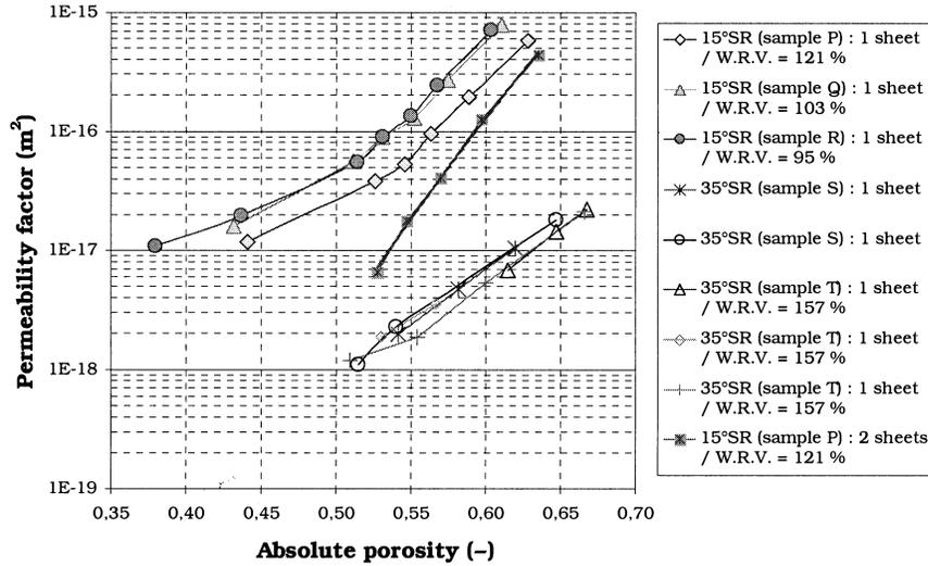
Figure 6. Results obtained with the PTP for samples made on a pilot paper machine for different conditions of pressing (initial dryness for samples P, Q and R are respectively 43, 48 and 50 % and basis weight for all the samples is 100 g · m<sup>-2</sup>).
