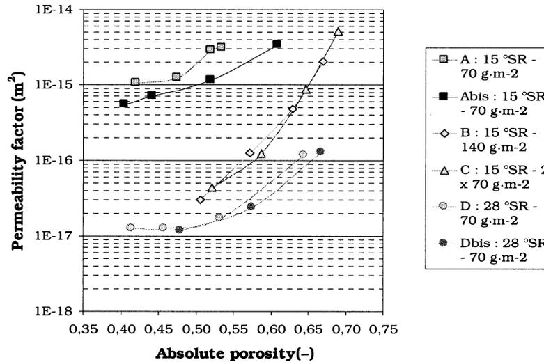
Figure 4. Results obtained for different handsheets with the PTP (beaten and unbeaten softwood webs).
