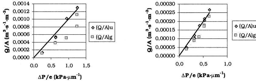
Figure 3. Examples of linearity (velocity,  $Q/A$  vs. pressure gradient across the sample,  $\Delta P/e$ ) and repeatability for two different sheets ( $Q$ : flow rate;  $A$ : area;  $\Delta P$ : pressure drop;  $e$ : thickness).
