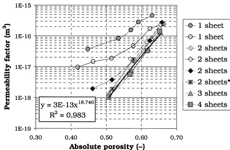
Figure 5. Results obtained for different stacked samples (softwood pulp; 80 g·m<sup>-2</sup>) (for the trial “2 sheets”, the sample was changed for each level of porosity).
