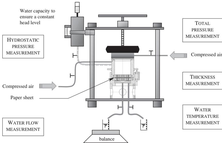
**Figure 1.** Schematic view of the Paper Transversal Permeability (PTP) device.
