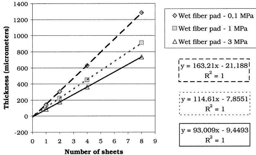
Figure 2. Example of linear relationships between thickness and number of sheets introduced in the cell.
