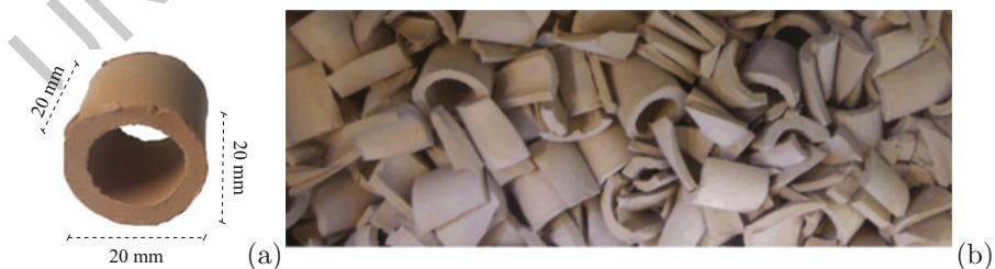
Fig. 1 (a) An intact shell (backed clay), (b) broken shell after an oedometric compression, \sigma_a = 420 kPa
