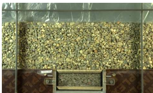
Figure 2. Picture of the central part of a test under cyclic load (trap-door replaced by foam element)
