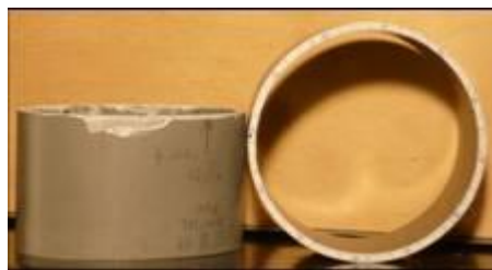
(a). Flexible PVC pipe; d=10.0\text{cm} , t=0.33\text{cm}
