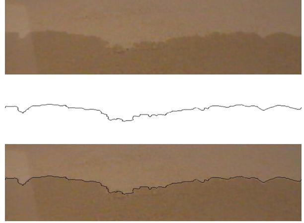
**FIGURE 2.** Image treatment of the air/liquid interface. The top panels shows the image captured from the digital camera, which was treated with ImageJ<sup>TM</sup> in order to obtain a single valued function, shown in the middle panel. The bottom image combines the single value function and the original image to compare the efficient of the procedure.
