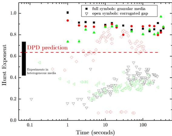
**FIGURE 4.** Time evolution of the Hurst exponent for the air/liquid interface in the displacement of air by water into granular media (filled symbols) or in the gap of two corrugated plates (open symbols). Three runs of each experiment is shown to facilitate the comparison. The value of  $H$  predicted from DPD model is indicated with a dashed arrow, and the range of experimental results is marked with a gray rectangle.
