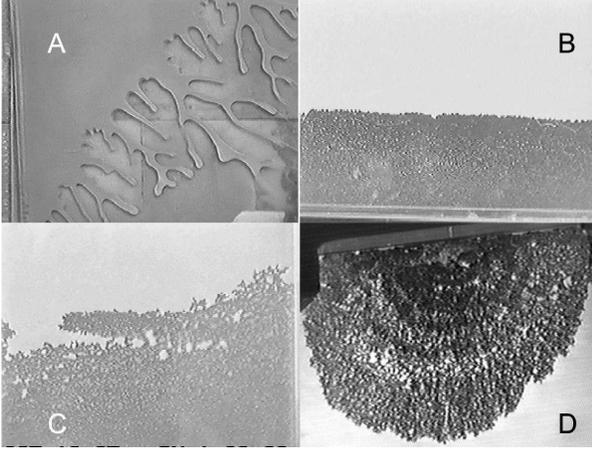
**FIGURE 1.** Fluid displacement in heterogeneous media. Examples of fluid displacement: (A) air displacing a moisture of glass, aluminum oxide and water; (B) and (C) water invading a narrow gap between corrugated plates at two different gradings - 80 *ppi* and 350 *ppi* respectively; (D) India ink displacing air in a 500 *ppi* corrugated channel, towards the direction of gravity (downward).
